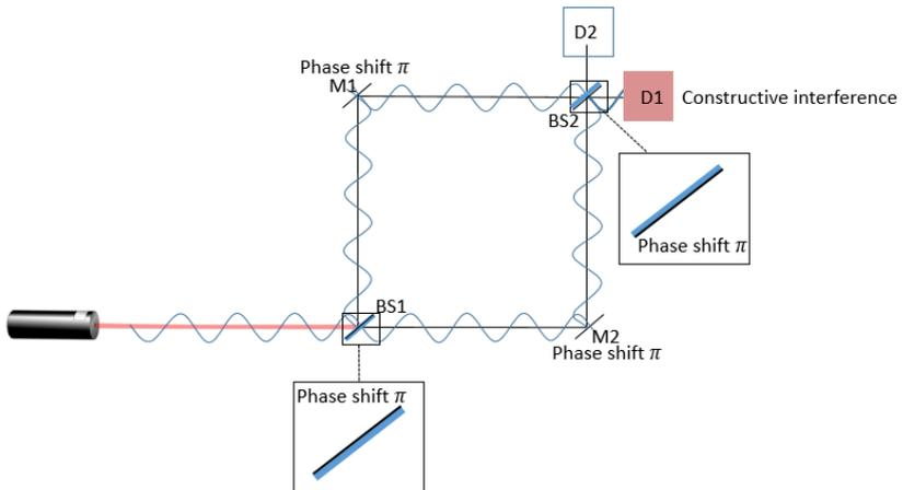
Figure 1.3: MZI with light beams. Constructive interference of subbeams A2 and B1 between BS2 and D1.
