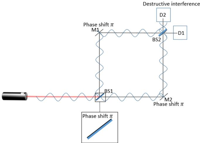
Figure 1.4: MZI with light beams. Destructive interference of subbeams A1 and B2 between BS2 and D2.
