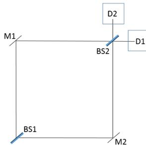
Figure 1.1: Mach-Zehnder interferometer (MZI).
