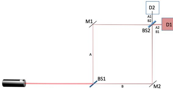
Figure 1.2: MZI with light beams.
