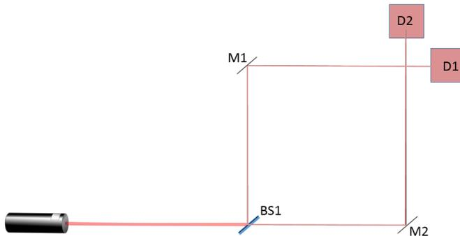
Figure 1.5: MZI without the second beam splitter BS2 and with light beams. Both detectors respond.
